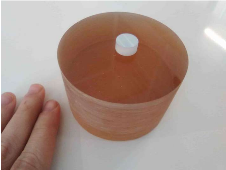
Figura 10: A very flat mirror (below) and a really flat mirror (on top).
